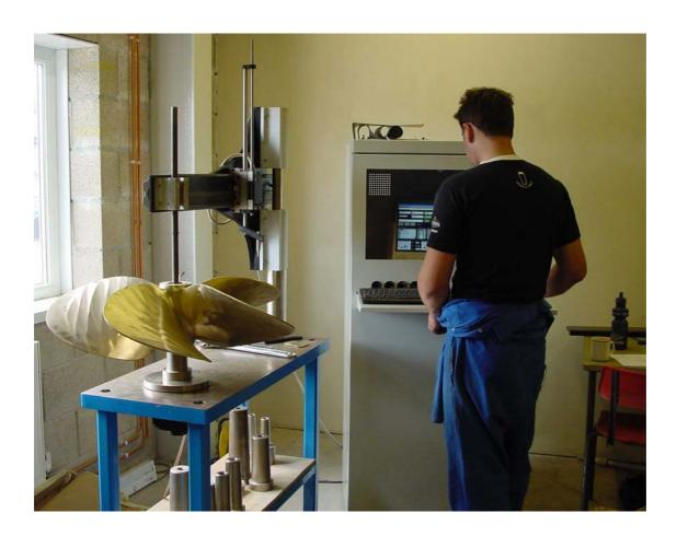
Propellers are inspected using computerised specialist measuring equipment to ensure conformity to propeller inspection standards.
