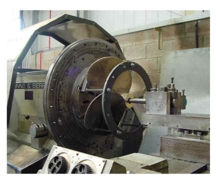
The company produces propellers up to 2.5 metres in diameter, propeller shafts up to 150mm diameter, and a variety of rudders shaft brackets and stern-gear components. These components are machined by highly skilled and trained staff using precision machine tools, special purpose equipment and C.N.C machines.
